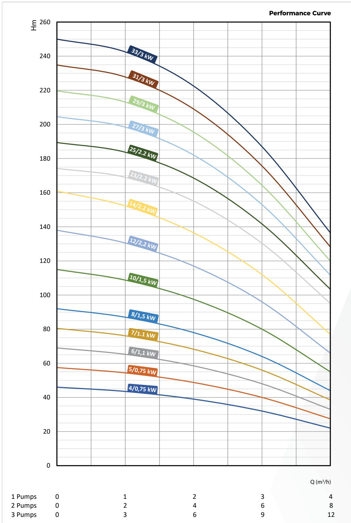
\*\*Frequency controlled panel on motor between 0.75 kW - 7.5 kW is used.\*\*
